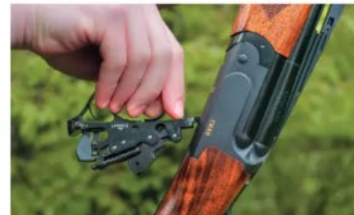
All CRX9 models come with a detachable wigger whose parts are all well finished
